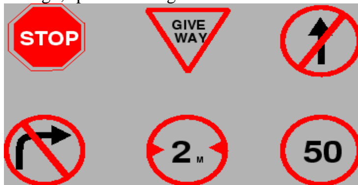
Fig. Examples of regulatory signs ( stop sign, give way sign, signs for no entry, sign indicating prohibition for right turn, vehicle width limit sign, speed limit sign)
