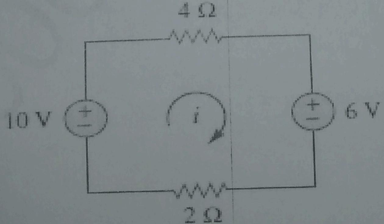
Find out (i)current (ii)voltage drop across 4 ohm and 2 ohm (iii) Power absorbed by resistance 4 ohm and 2 ohm.
